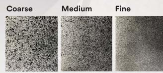
\* Results above created with 3M<sup>™</sup> Waterbased Undercoating, PN08881
