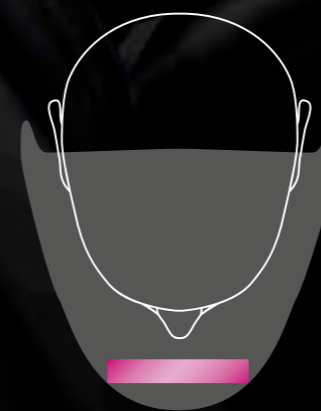
Flat ADF in a slim helmet means the ADF can't be wide.
