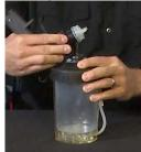
8) Attach the loose end of the air hose to the H/O conversion Pack supply port
