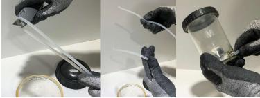
7) Attach to the cup to the Performance Spray Gun nozzle before inverting the cup
