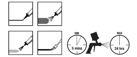
3M<sup>™</sup> 50740 Beige hybrid sealant is a sprayable sealant in cartridge for general purpose from the formulation of a hybrid polymer (no isocyanates). Packaged in aluminium cartridges of 310 ml
