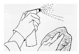
4. To minimise clean-up of film remover the following method should be used: Mask the surface around markings and make a 'drip trough' with masking tape or cardboard to prevent residue dripping onto surfaces around the marking.
