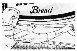
5. Make certain that the application surface temperature is at least 10°C (50°F). If it is 29°C (85°F) or above, move the vehicle to a shaded area and allow to cool down.
