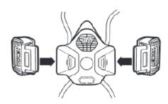
HF-800 Series Half mask and associated filters have an inhalation breathing resistance of less than 5 mbar, when measured at 95 lpm continuously.
