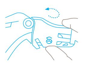
**Close** the blade cover and **fold the blade carrier back** into the handle letting the blade change button **audibly snap** into place.
