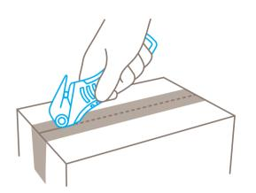
To use the **adhesive tape splitter**, turn the cutting tool around by 180 degrees.
