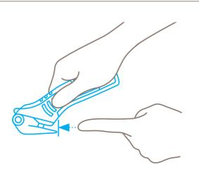
The concealed blade provides a maximum degree of **protection from cut injuries**.
