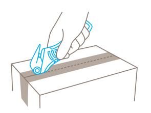
To use the **tape splitter**, turn the cutting tool around by 180 degrees.
