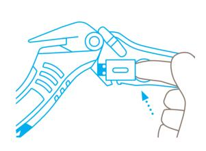
Place the thumb on the blade symbol and open up the blade cover. Remove the blade from the **side**. Turn or change the blade.
