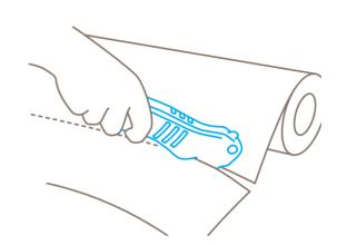
When cutting film and paper, ensure the material to be cut is under **tension**.
