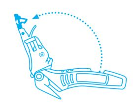
**Fully** open the blade carrier from the handle using the blade change button.
