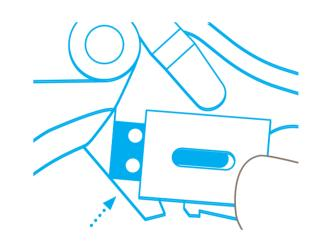
Then align the blade **to the left edge** and insert exactly onto the locating lugs.
