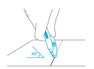
Hold the cutter at a **slight angle** when cutting through cardboard boxes.
