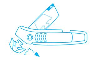
Position the spare blade **parallel** to the slanted side of the cutter head. Push the blade in, and then **downwards**, until fully engaged.
