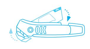
Push the blade magazine back into the han**dle** to lock the blade head in place.
