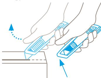
**Automatic blade retraction – a high degree of safety**
