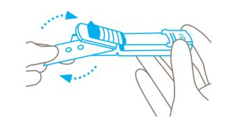
Reverse or replace the blade. Make sure you place the blade **exactly on the locating lobes**.
