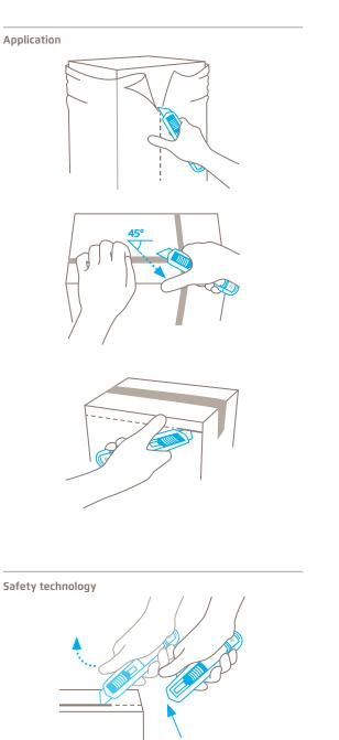
Automatic blade retraction – a high degree of safety The automatic blade retraction of the SECUNORM 525 guarantees a high degree of safety from cut injuries. As soon as you have started to cut, take your thumb off the slider. Then the blade will retract into the handle immediately after leaving the material being cut.
