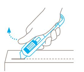
Always remove your **thumb from the slider** to ensure automatic blade retraction.
