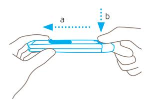
Close the blade cover and push the plastic insert back into the handle and then **press** down on the blade change button.
