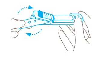
Reverse or replace the blade. Make sure you place the blade **exactly on the locating lobes**.
