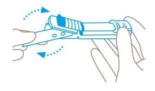
Reverse (for left handers) or replace the blade. Make sure you place the blade **exactly** on the locating lobes.
