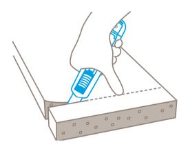
For thicker material, position the blade at a 60° angle to take full advantage of the cutting depth.
