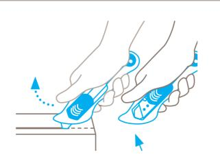
Following cutting, the blade immediately retracts into the handle. Condition: you have released hold of the slider.
