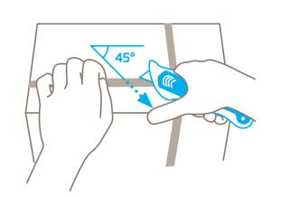
Use the slider to **engage the blade** for cutting.
