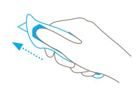
Change the blade from the front side. Simply **lift** the slider and carefully remove the blade.
