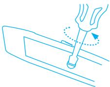
Unscrew the handle and remove the upper half of the handle. Reverse or replace the blade.
