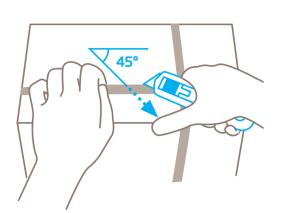
Use the slider to **engage the blade** for cutting.
