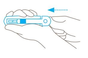
Use the slider to **push** the plastic insert back and out of the handle. Don't pull the insert while holding onto the slider.
