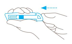
Use the slider to **push** the plastic insert back and out of the handle. Don't pull the insert while holding onto the slider.
