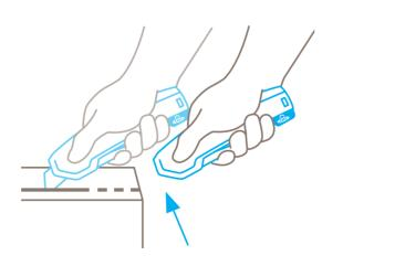
The blade immediately retracts into the handle the moment cutting ceases. Even when the lever is **still being squeezed**.
