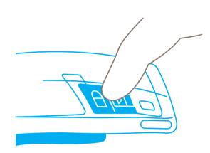
To prevent unintentional blade activation, always **lock the cutter** by pressing downwards on the lock symbol.
