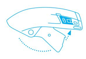
Finally, push the lever back into the handle until you **hear it click into place**.
