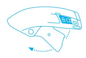
**Swing the lever out** of the handle and flip open the blade cover.
