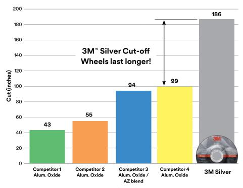
Internal 3M testing on 304L stainless steel sheet (11 gauge) using a 13 amp electric tool. Wheels are tested to end of life.
