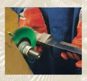
■ **Light Deburring** - The Radial Bristle Brush deburrs quicker and more effectively than wire or nylon brushes, leaving a totally burr-free surface.
