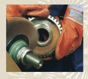
■ General Cleaning - Radial Bristle Brushes are an excellent tool for general cleaning and finishing on a variety of metals, without removing base material, reducing the chances of damage or reworking.
