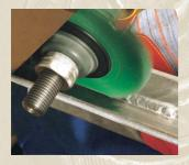
■ Weld Cleaning - Especially on stainless steel the product gives an excellent finish, quickly, with no smear, even when the work-piece is hot.
